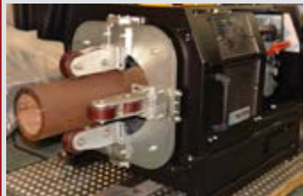
OHSB Beveling Machines for Very Heavy Wall Thicknesses
