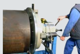
US450 Heavy Duty Beveling Machine for Large Diameters
