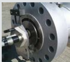
Facing and Machining Flanges and Valves
