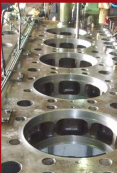
Machining 6 cylinders + positioning inserts in ten days.
