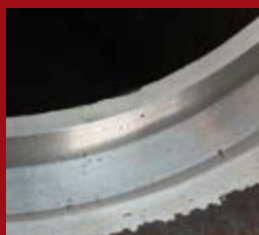
Conical machining – RTJ (23°) or any other angle (30°, 45° etc.)
