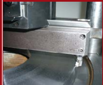
Machining RTJ groove bearing surfaces
