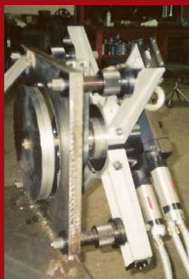
Trepanation of sheet metal up to 50 (1.968") mm thick
