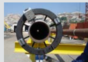
TT-LW Light Weight Orbital Pipe Cutting Machine
