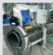
TNO Orbital Cutting and Beveling
