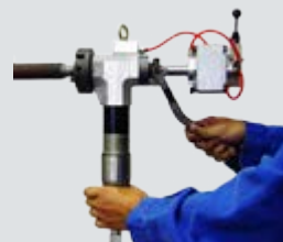
Machines for US-CA / US TP Heat Exchanger Tubes
