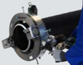
TT-NG Orbital Cutting of Thick Wall Pipes
